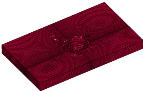
Figure 5. Crater created in the soil from the explosion and soil ejected in the air
